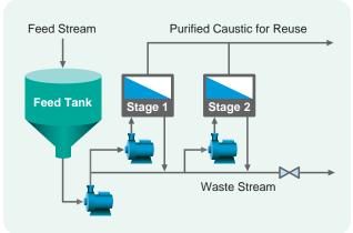
In this mode of operation, feed is directly pumped into a baseline pipe and recirculated through two stages of membranes. Clean permeate is produced at a steady flow rate and quality, while the process parameters are automatically controlled.
