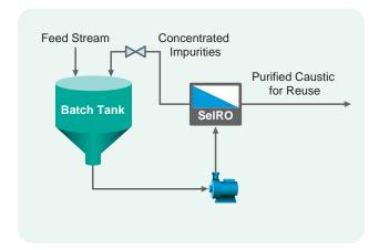
The Causti-COR system treat the contents of a batch tank. Purified caustic solution leaves the system, while concentrated impurities return to the feed tank for reprocessing. When the desired product recovery is achieved, the batch tank is drained and refilled with fresh feed.
