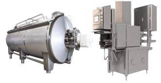
RELCO technology provides efficient and sanitary handling and packaging of various powders. Our powder handling and packaging systems transport, discharge, fill, weigh, blend, and package powders with consistency and reliability.
